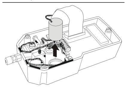
Figure 6-3 Removing a Sensor from the Innova
